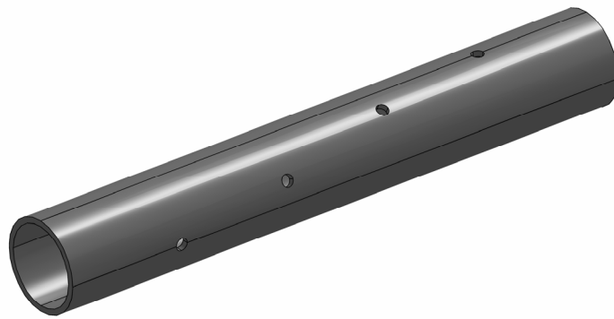
Figure 2. Test pipe with 4 shifted artificial defects
